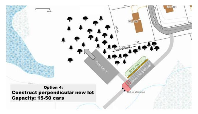
Utilizing the sparsely-wooded area behind the kiosk would allow a second lot to be installed. There is plenty of room for a significant lot (survey needed to determine wetlands, etc.). The woods between the expanded lot and the abutter are dense enough to provide visual shielding. Could be combined with most other options, but not really needed. Note loss of 2 original spaces.
