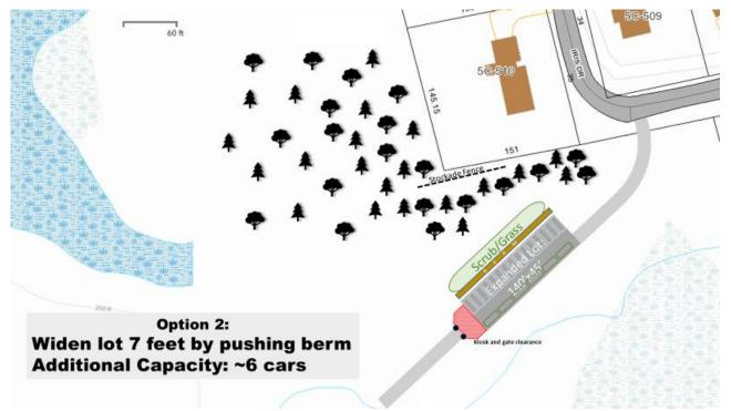
Pushing the berm about 7 feet back would allow 6-7 cars to park safely on the left side, easing backing-up and allowing fire lane access. This would not affect sight-lines to the abutter. Combining with option 1 adds another 5-6 spaces.
