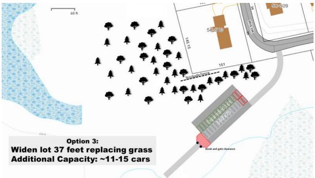
Using most of the existing berm and grass space would allow the lot to be expanded to about 75 feet in width, allowing two rows of cars to park nose-in. Accommodation for cars to drive to the other side will be needed (remove 1-2 spaces each row; could extend lot toward Currier Rd to alleviate this)
