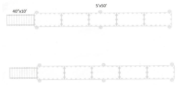
Each dock shall consist of 5 sections which are a minimum of 10 feet long x 60 inches wide. In addition there will be a ramp from the shore to the dock which is a minimum of 10 feet long x 40" inches wide. Each separate floating dock should include a swim ladder and appropriate hardware to attach to the dock.
